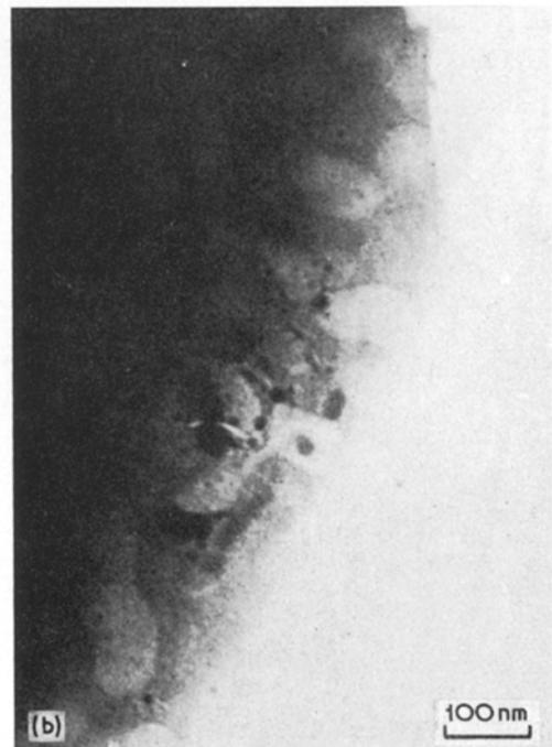
Figure 9 Transmission electron micrographs of specimens of composition 10 Na<sub>2</sub>O, 10 CaO, 80 SiO<sub>2</sub> (mol %) ion-exchanged at 600°C for 1 h after various heat-treatments. (a) As-cast, (b) heated at 660°C for 16 h.
